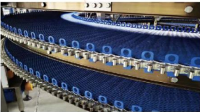
Food-Grade High-Strength Plastic Conveyor Belt
